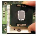
Align pin 1 of processor with pin 1 of the CPU socket.
